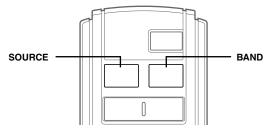
2 Press the BAND button on the CDA-9807/CDA-9805 or the RUE-4187 to activate the CD Changer Selection mode. 3 The CD Changer Selection mode remains active for 8 seconds after step 2 is performed. Press the BAND/ TEL. button until the desired CD Changer indicator appears on the display.
